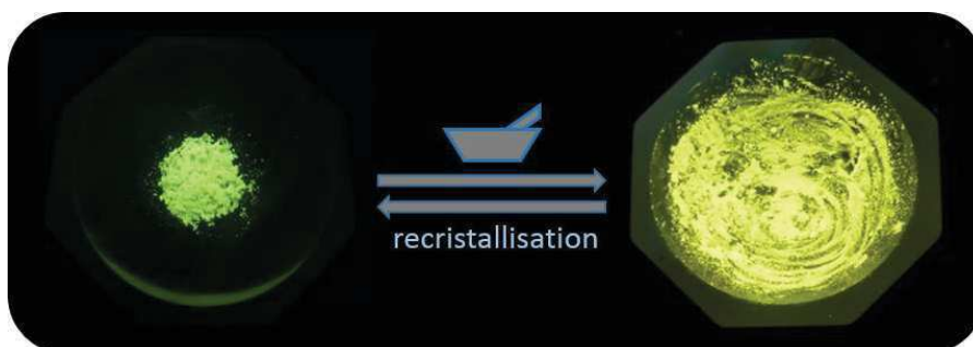
Figure 1. Luminescence mechanochromism of a [\text{Cu}_4\text{I}_4\text{L}_4] (L = phosphine ligand) cluster.
